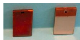
Figure 3. Control copper substrate (left) and copper with 11 monolayers of C18N in LB film (right)
